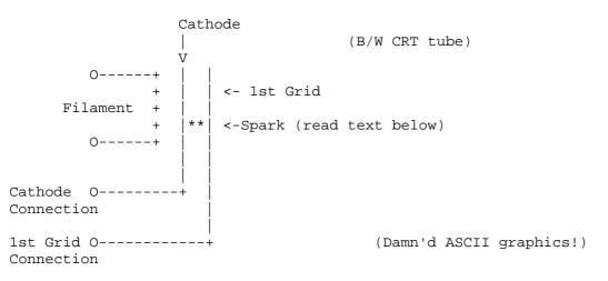
Try to connect and turn on the transformer. The Filament in the CRT should turn on in a notso-bright red (if it is a colour tube, we have 3 filaments on).
