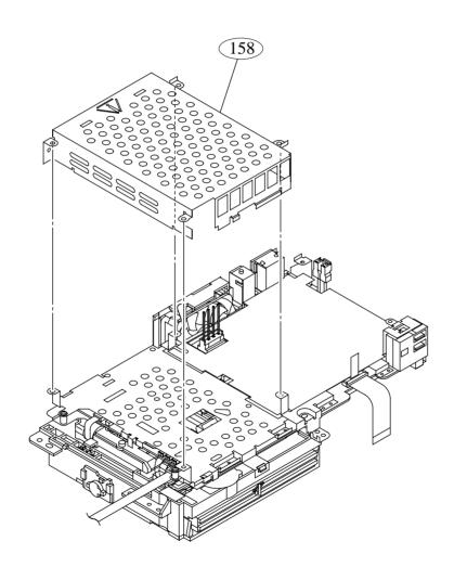
Never lose the fitting of INSULATING SHEET put on the SHIELD(B) when assemble the console.
